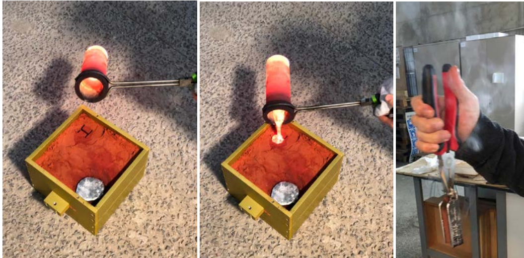
Figure 2: Aluminum pouring into sand mold
