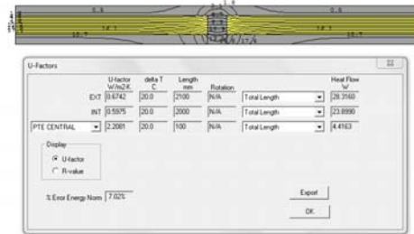
Fig. 1: Example of thermal bridge simulation with Therm
